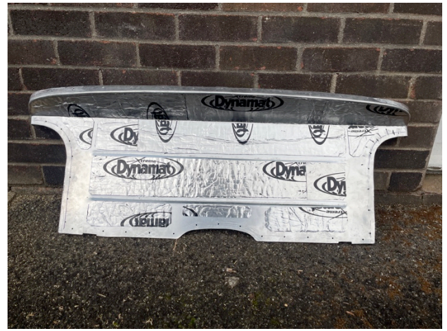
Firewall with Dynamat ready for fitting
