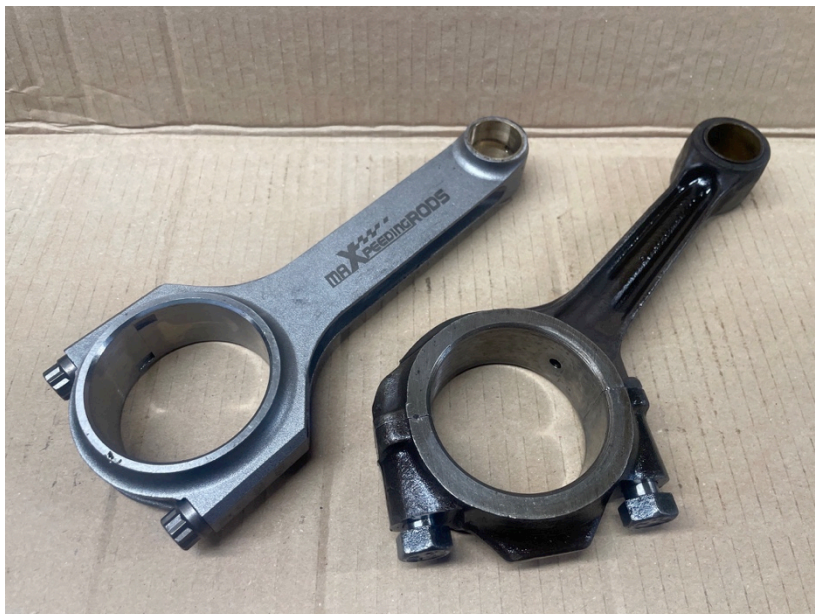
The new forged conrods are balanced to within 1g, weigh around 2/3 the weight of the standard item and are much stronger.
