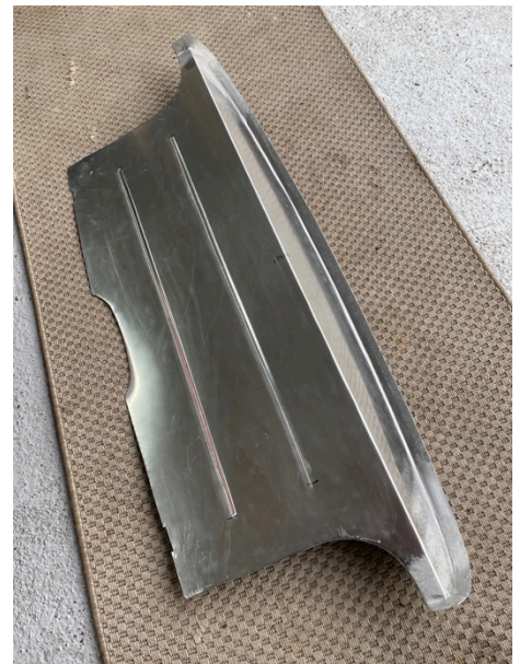
A couple of bead rolled flutes stiffened the flat panel.
