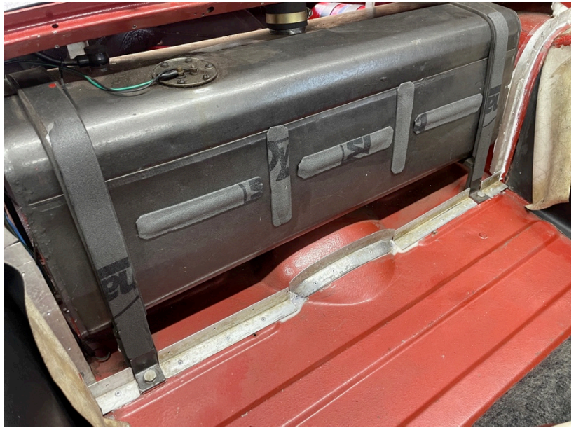
Angle frame in place with strips of Dynaliner on tank and straps
