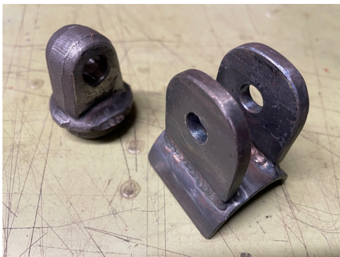
A forged OMP lug with the home fabricated fork.
