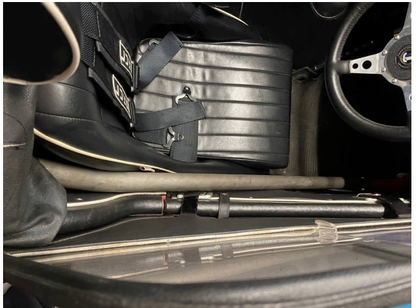
Routing past the seat, avoiding the door and side-screen mounts is tight.
