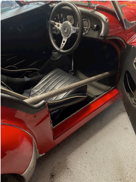
The drivers-side door bar mocked-up in place.
