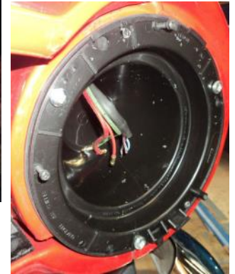
TR6 replacement headlight bowl with rim retaining lug.
