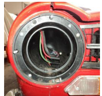
TR6 headlight bowl , no retaining rim securing lug
