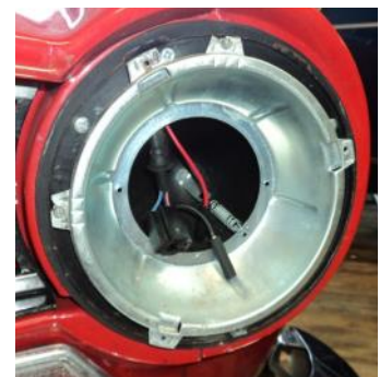
TR6 headlamp bulb with adjusting inner facility
