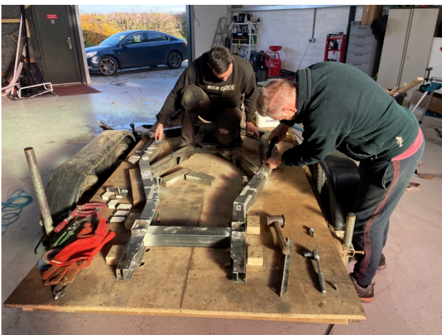
The chassis being fitted and aligned in the jig.
