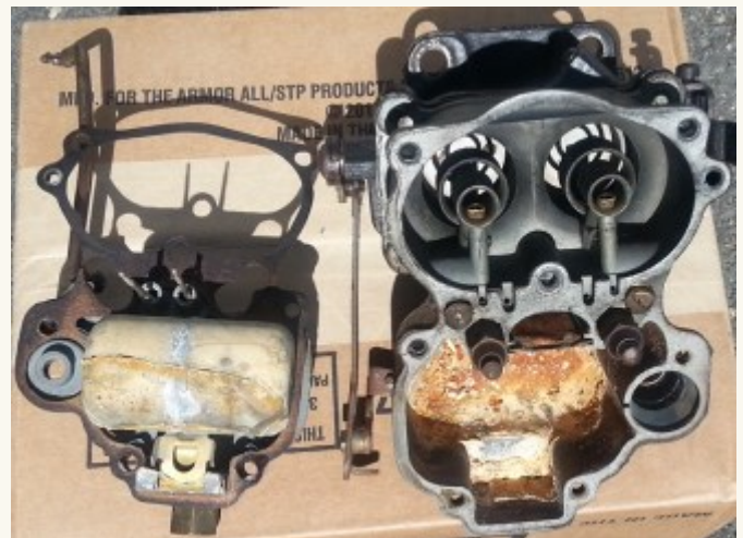
Fig 1. Corrosion in the float chamber caused by untreated E10 petrol & water.
