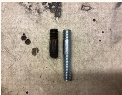
Fig 2— old and new studs
