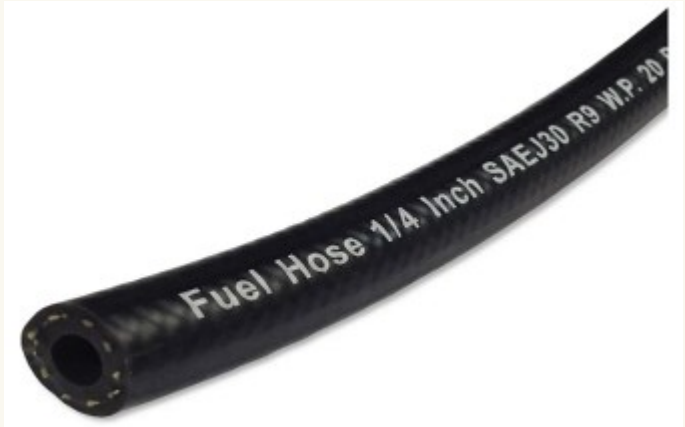
Fig 3 SAE J30 R9 ethanol compliant fuel hose showing the correct identification including the working pressure which in this case is 20 bar or 290psi.
