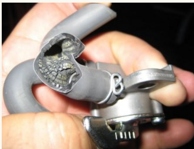
Fig 2 Effect of ethanol on an incompatible fuel pipe material
