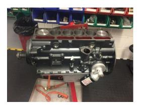
The engine is starting to look slightly more like an engine at this point as we flip it over and add a few bolt-on ancillaries such as the oil filter. We give the crank a few gentle turns to make absolutely sure there are no suspect noises of catching, and turn our attention to the Head.
