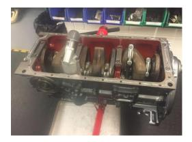
Once the timing chain was sorted, it was time to cover it up. As some of the same bolts hold the timing cover on as hold the engine plate on, these need to be removed, Loctited, and replaced, not forgetting to include the alternator mount and the timing cover oil seal. The oil pump is then checked for tolerance (0.002"!), primed with Vaseline and fitted "hard hand tight". Then the sump cover is fitted with sealer, remembering the front 2 and back 3 bolts are shorter than the rest.
