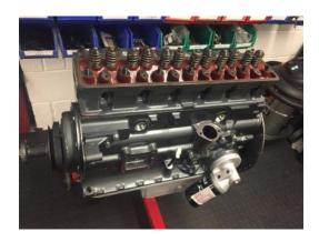
A composite gasket was used between the block and the head which meant no sealer was needed. A light coating of assembly lube was added to each stud to avoid binding and the head was placed very carefully over the studs. Washers were coated with torque fluid above and below and torque fluid was also added to the stud threads. Nuts were cleaned and Added. The head was then torqued down in three stages, following the correct pattern and procedure for tightening the nuts:
