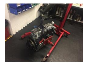
Various tasks were completed following this point. This included fitting the flywheel, oil pressure relief valve, clutch plate (using alignment tool), water pump (not forgetting the alternator bracket), thermostat and cover, oil pressure warning lamp sender. The engine was then removed from the engine stand and that day's work was complete.
