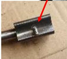
obviously been working its way loose for some time including during a 3,000 mile road trip to Italy. Eventually, in Scotland, the pin finally worked its way to the point that it locked up and the pump stopped working.
