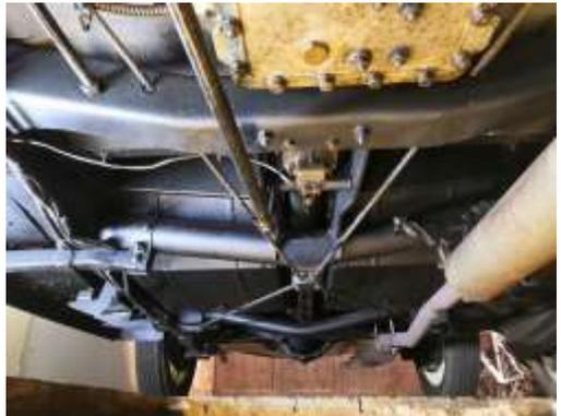
Photo of the underside of the Riley - note the cable tensioners to stiffen the chassis.
