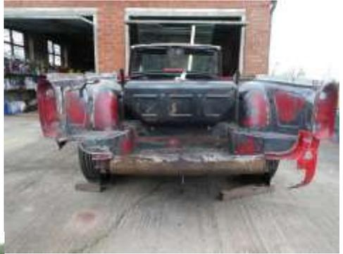
Although some work had been done to the chassis, the body was dismantled revealing lots of rot and bodged repairs so he had plenty of work cutting, welding and fitting replacement panels. Phil has converted her to right hand drive and she is full TR 5 spec now. At some point she had been resprayed red but Phil decided revert to the original green.
