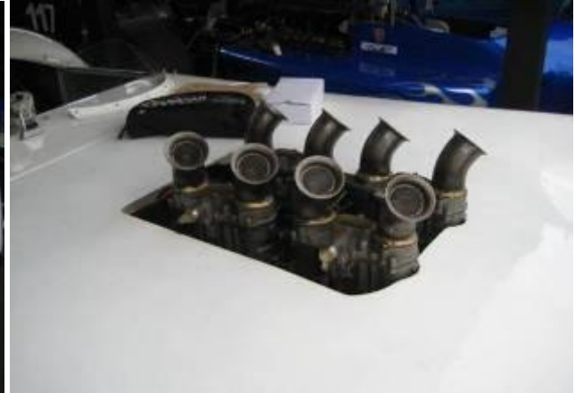
Chapman Mercury 3 4700cc with intake trumpets angled to benefit from forward motion....!!
