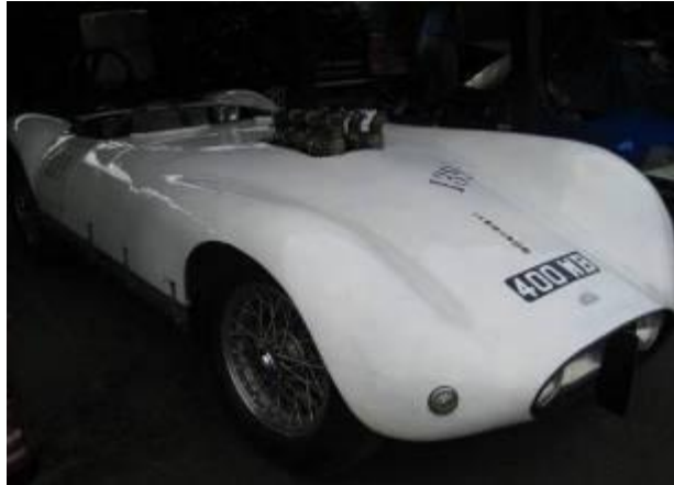
Chapman Mercury 3 4700cc with intake trumpets angled to benefit from forward motion....!!
