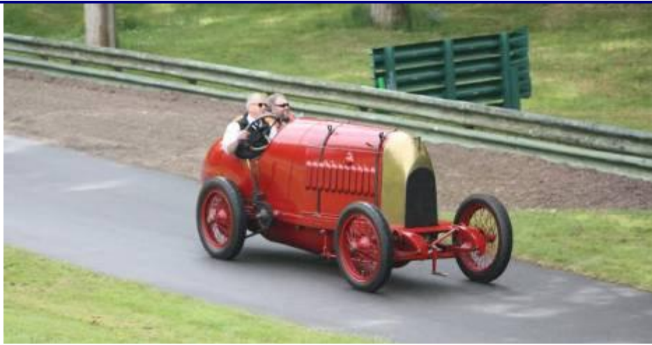
The 'Beast of Turin' this 1910 Fiat was built to challenge the World Land Speed Record, this monster was propelled by a 28.5 litre aero engine producing 300 bhp at 1800rpm capable to to propel this 'Beast' to 116mph and achieve a one mile land speed record in 1911. Driven here on a demonstration run by its restorer and owner Duncan Pittaway. Loads of information on the internet relating to this engineering monster.
